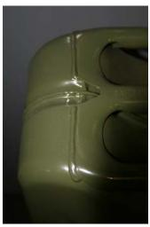
Strip welded handles tested to hold 24 kilo's of weight when dropped from 1.8 metres
