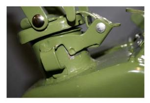
Lid moves freely in vertical motion, reduced sealing ability.
