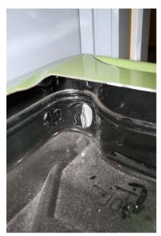
Welded areas melt internal paint and leave exposed bare metal.
